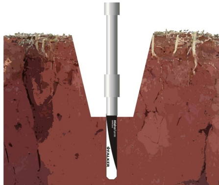
Figure 9: Sensor installed in the subsurface of the floor together with the extender after opening the trench
